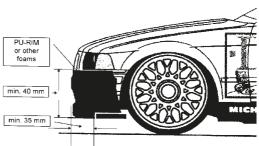
no point may any part of inflexible material for bodyshell mounting protrude from the body more than 10mm. If an opening is created through the foam bumper for cooling air, the combined thickness of the foam (above and below the cooling hole/slot) must still be a minimum of 40mm in height.
